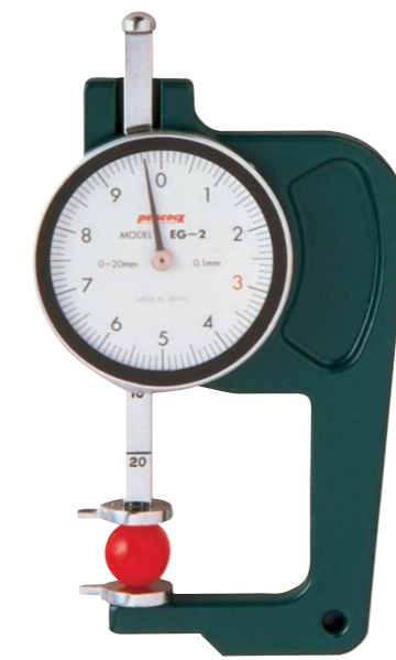
EG-2 for measurement of inner diameter, outer diameter and depth.
